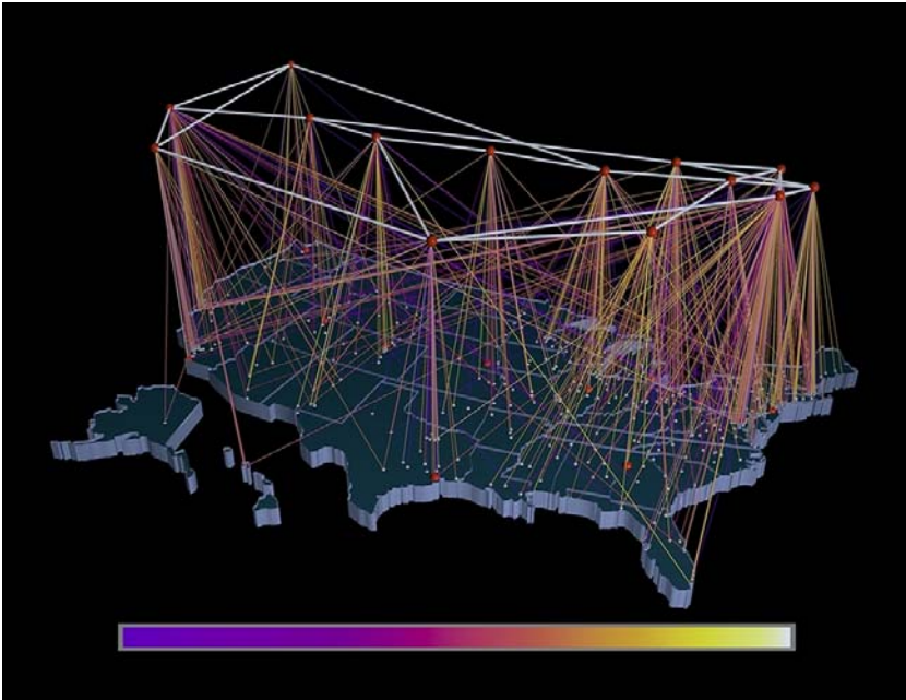
Fig. 5.9 An image that shows the topology of the NSFNET T1 backbone network in September 1991 in the United States. The situation today is certainly more complex than that represented in the figure. Created by D. Cox and R. Patterson/NCSA, UIUC. © 1994 The Board of Trustees of the University of Illinois.
